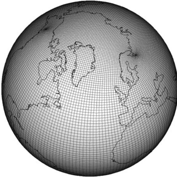
Fig. 16.3 The tripole grid used by POP. The coordinate seam in the tripole grid connects a pole in the Yukon Territory of Canada to one near Arkhangelsk, Russia
