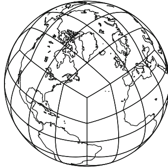
Fig. 12.2 Tiling the surface of the sphere with quadrilaterals. An inscribed cube is projected on the surface of the sphere. The faces of the cubed-sphere are further subdivided to form a quadrilateral grid of the desired resolution. Coordinate lines from the Gnomonic equal angle projection are shown
