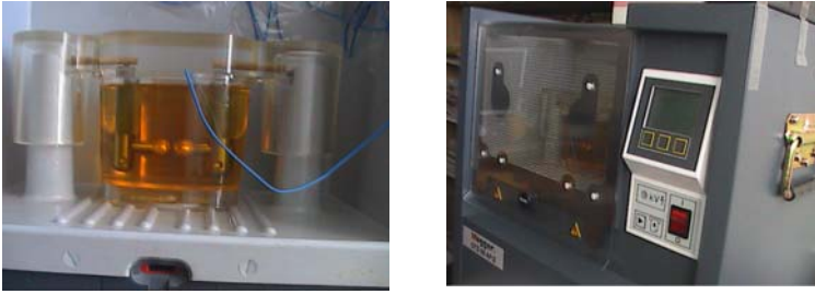
Fig. 1. Equipment for oil electrical breakdown testing
