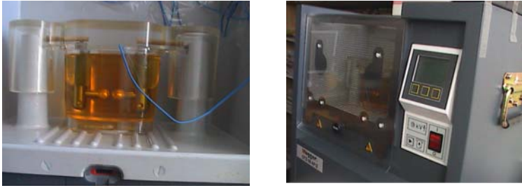
Fig. 1. Equipment for oil electrical breakdown testing
