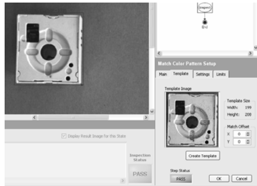
Fig. 2. Match Pattern Color Vision Tool setup
