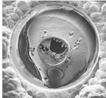
Fig. 6. The obstruction has fallen out of the flexure
