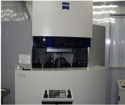
Fig. 1. Image of the Zeiss F25 CMM, located in the PMC facilities
