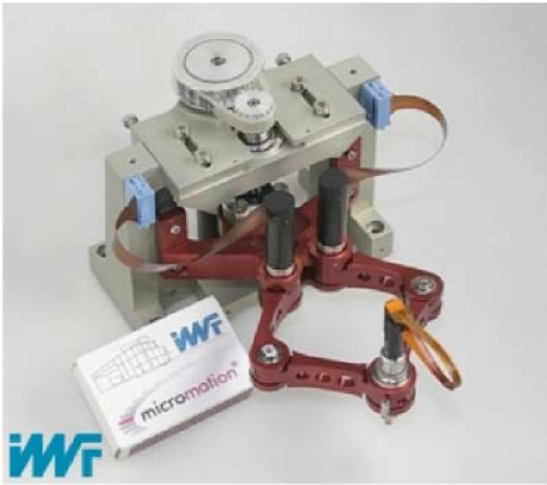
Fig. 1. PARVUS parallel scara-robot [4]
