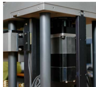
(b) AC servo motor is attached to gear driven structure
