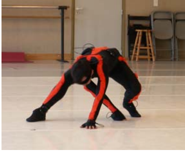
(a) Affective dance collection: the Dancer wearing the Moven motion capture suit
