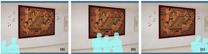
Fig. 1. Scenario of the uPoster. (a) Ladies are animated while there is on one around. (b) Ladies are static while people walk into the detecting area of web camera. (c) Ladies are playing again.
