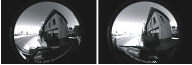
Fig. 7. Stereo pair of fish-eye images, for ensuring a wide field of view in vision based driver assistance
