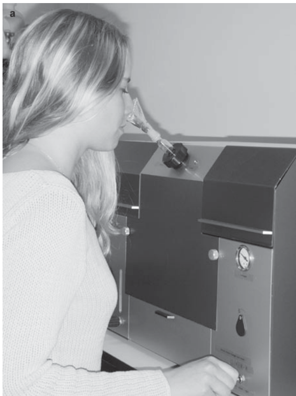
Fig. 19.2 Measurement of the threshold level of vanilla with an olfactometer
