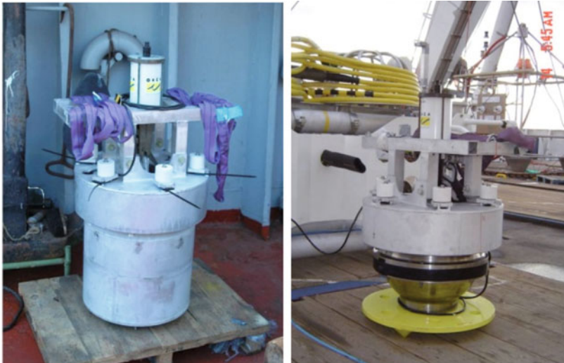
Figure 11.8 Seismometer management systems (left) used in GEOSTAR, SN2, SN3 and SN4; (right) used in SN1.
