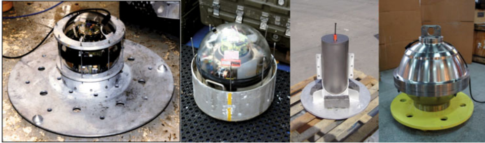
Figure 11.7 Different arrangements for the seismometer. From left to right: Guralp seismometer first arrangement (GEOSTAR mission 1); same instrument with an upgraded arrangement (GEOSTAR mission 2 and SN1 first mission); arrangement for PMD seismometer (GEOSTAR missions 3 and 4, SN2 mission 1, SN4 mission 1); Guralp seismometer final arrangement in titanium sphere (SN1 missions 2 and 3).
