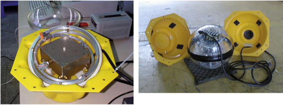
Figure 11.5 Gravity meter (left) during customization work and laboratory tests; (right) Vectorial magnetometer integrated into a glass sphere.
