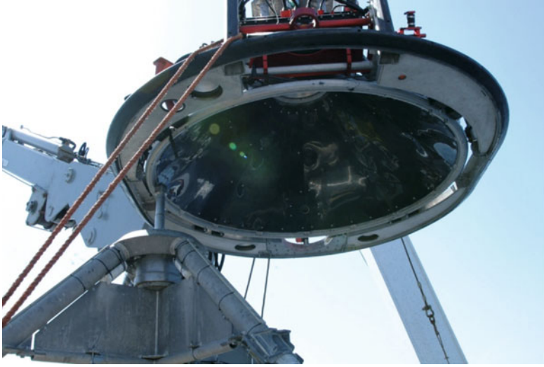
Figure 11.10 GEOSTAR–MODUS connection principle, based on docking pin (on GEOSTAR) and latching device (on MODUS).
