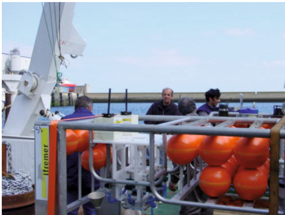
Figure 9.5 Messenger rack on Station-1. Station-1 was equipped with an 8-slot Messenger rack. Main characteristics: height 480mm; tube diameter 38mm; buoyancy block 150 × 150 × 150mm; mass 32 kg; buoyancy 0.6 daN.
