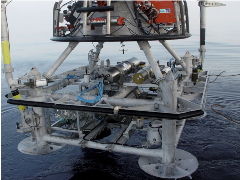
Figure 11.4 Typical GEOSTAR mission setup; note the payload arrangement on the open frame.
