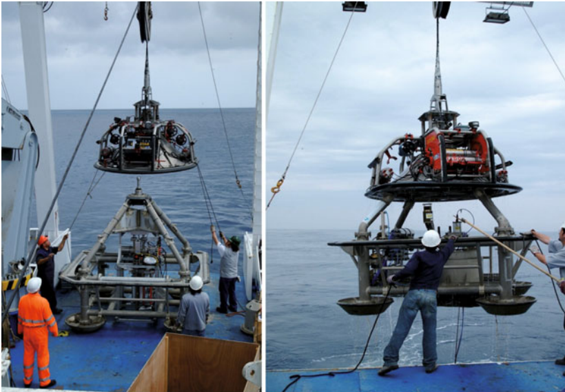
Figure 11.44 Comparison between SN3 configurations; (left) with ASTRA; (right) with a standard seismometer.
