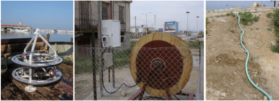
Figure 11.56 (Left) GMM ready for deployment in Patras Gulf; (center) Shore Unit; (right) umbilical cable.
