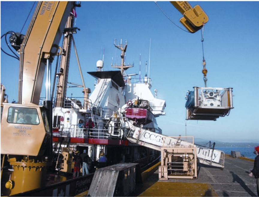
Figure 16.9 Instrument pod for test deployment in Saanich Inlet being loaded onto CCGS Tully.
