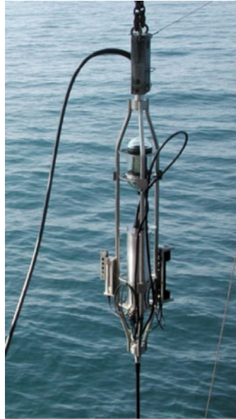
Figure 15.10 Storey 1 of MILOM line showing a CTD, a C-Star and an optical beacon.
