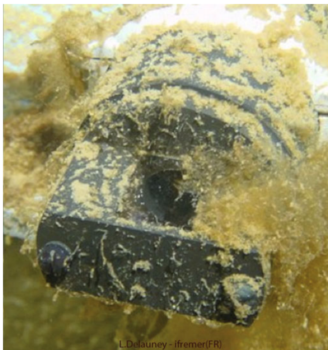
Figure 8.9 Fluorometer after 90 days in the roadstead of Brest (France) in the summer.
