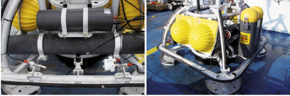
Figure 11.50 (Left) Methane sensors arrangement (the one fitted with a flow-through pump is visible on the right). (Right) Detail of the frame with two buoyancy spheres and recovery system based on a pop-up buoy and rope canister.
