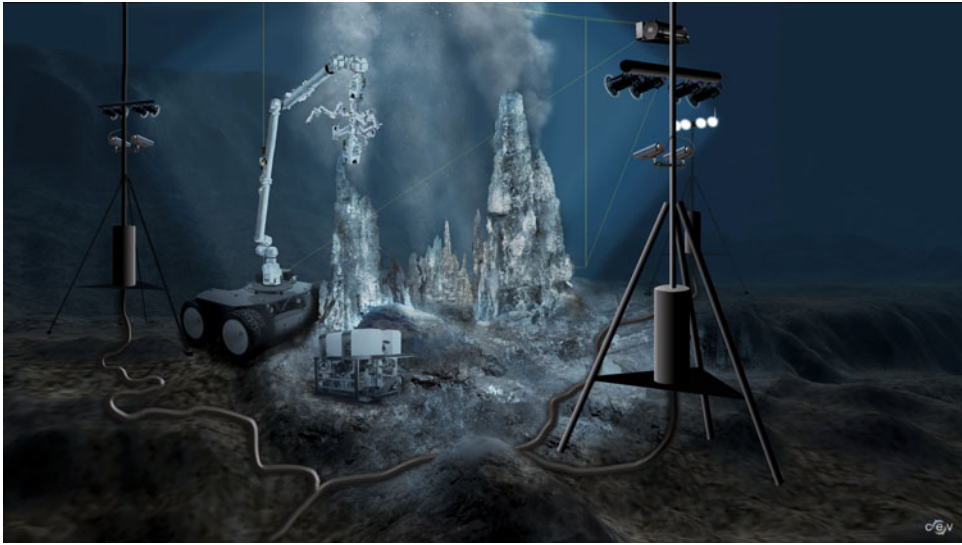
Figure 18.14 An artist’s depiction of a fully automated seafloor analytical laboratory within an active submarine hydrothermal system, operated serially or in parallel by different remote science groups on land using the power and bandwidth provided by industry standard electro-optical cables. Real-time analysis, in situ specimen dissection, and complex experiments can be conducted on materials flowing through the environment of this volcanically-driven ecosystem containing exotic microbial communities. Full operation of such an environmental laboratory will require integration of many emergent technologies. A system of this type, and a host of others, will become commonplace as the emergent technologies are increasingly integrated into next-generation forms of human telepresence in the oceans.
