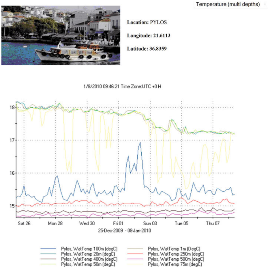
Figure 5.4 Example of the data viewing service offered by the POSEIDON web page ( www.poseidon.hcmr.gr ) displays the last 15 days' temperature time series at different depths from the POSEIDON-Pylos (Hellenic) observatory.
