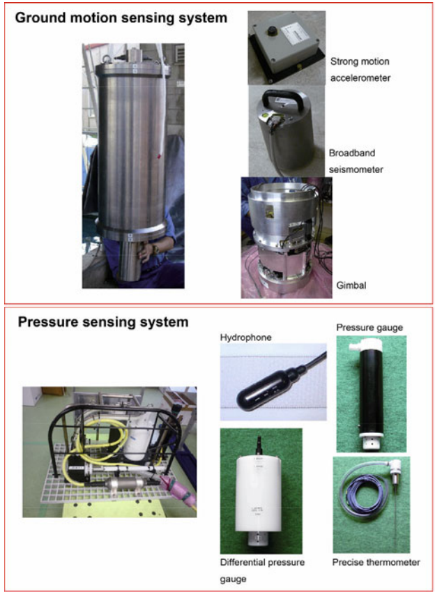
Figure 25.6 Sensors used by DONET system. (Upper) Ground motion sensing system. In a pressure-resistant case in the left, strong motion sensor and broadband seismometer attached on the gimbal mechanism. (Lower) Pressure sensing system. On the grating board, pressure gauge, differential pressure gauge, hydrophone and thermometer are attached.
