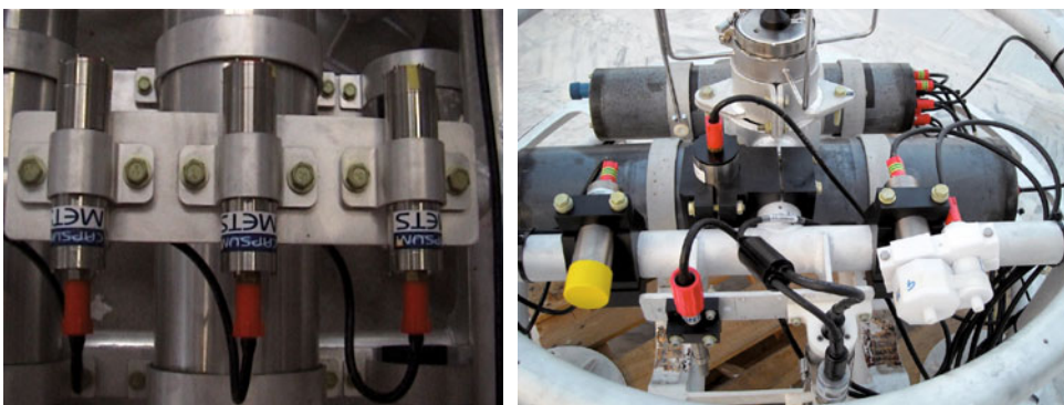
Figure 11.58 Comparison between methane sensor arrangement in GMM. (Left) 2004 configuration (three sensors in series). (Right) 2010 configuration (two sensors, of which the one fitted with flow-through system is visible on the right).
