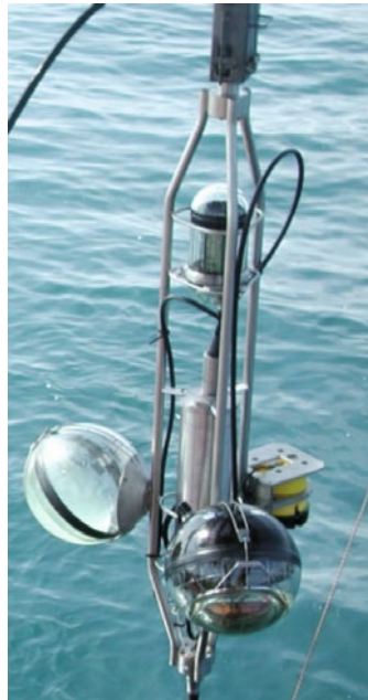
Figure 15.11 Storey 3 of MILOM line showing an ADCP, an optical module, a flotation sphere and an optical beacon.
