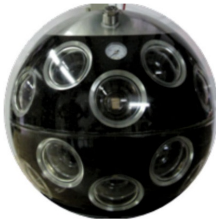
Figure 3.10 The KM3NeT Digital Optical Module (DOM) prototype (The KM3NeT Consortium, 2010).
