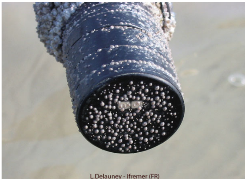
Figure 8.8 Turbidimeter probe after 14 days in Mont St.-Michel Bay (France) in the spring.
