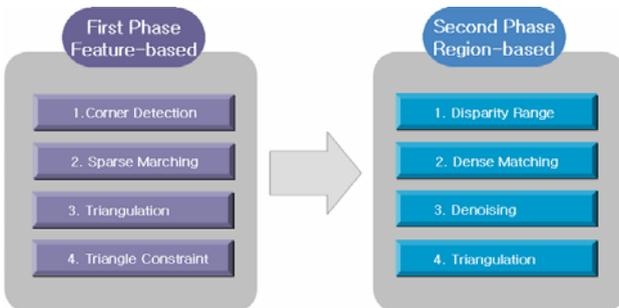
**Fig. 1.** Overview of the proposed stereo matching algorithm
