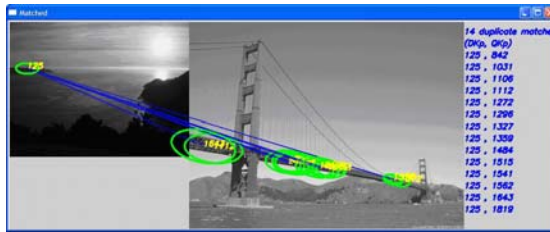
Fig. 5. Right: query image. Left: database image. Illustration of a typical problem of the matching algorithm: one keypoint in the database image has duplicate matches in the query image (14 matches in this example).
