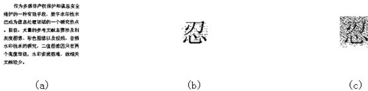
Fig. 8. (a) Watermarked image after 0.75-time scaling attack, (b) Extracted watermarking after scaling to the original size using usual DWT scheme, (c) Restored watermarking using dual watermarking scheme
