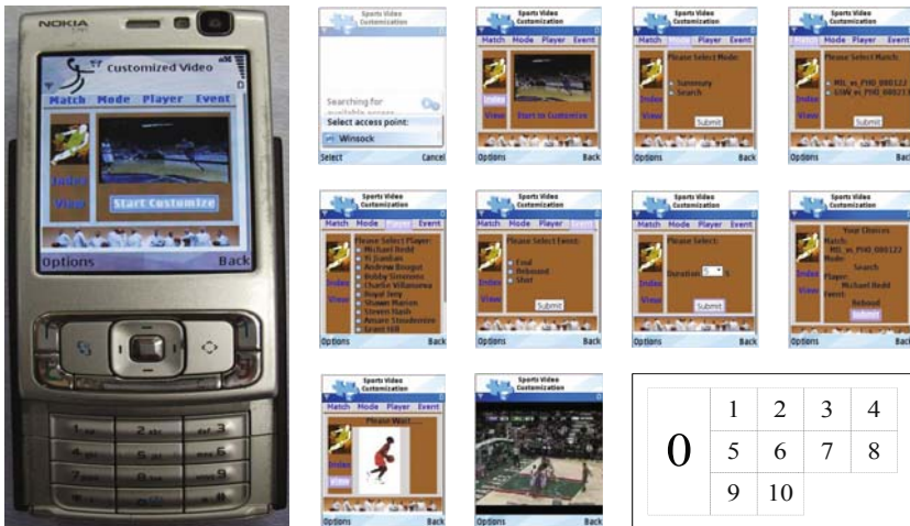
Fig. 5. The client interface on the Nokia N95 cell phone and a customization scenario example. (1) connect multimedia server; (2) enter customization user interface; (3) choose customization type; (4) choose match; (5) choose favorite players; (6) favorite event(s); (7) set viewing time; (8) request confirmation; (9) wait; (10) video playing.
