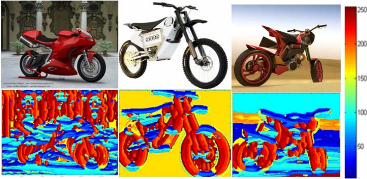
Fig. 3. Both image and BoWI with different viewangle and background are shown for the same bike object. Similar structure of the wheels and parts of the bike are not lost in the BoWI representation.
