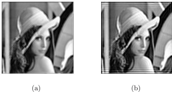
Fig. 5. (a): Deblurring result of traditional IBD method for defocus blur (b): Deblurring result of PSF-constraints IBD method for defocus blur
