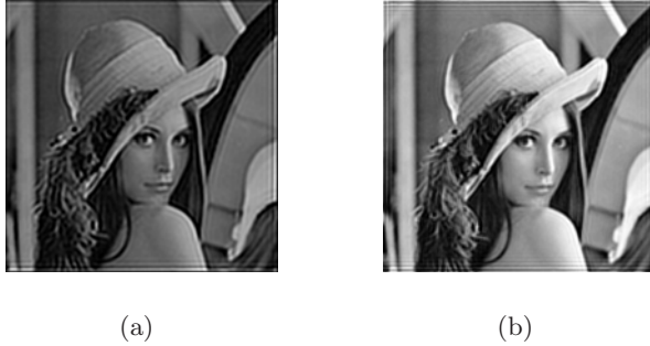
Fig. 7. (a): Deblurring result of traditional IBD method for gaussian blur (b): Deblurring result of PSF-constraints IBD method for gaussian blur
