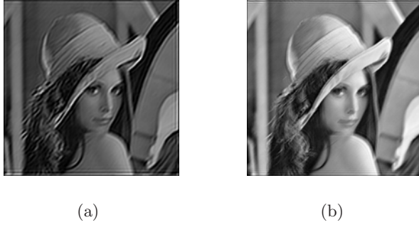
Fig. 3. (a): Deblurring result of traditional IBD method for motion blur (b): Deblurring result of PSF-constraints IBD method for motion blur
