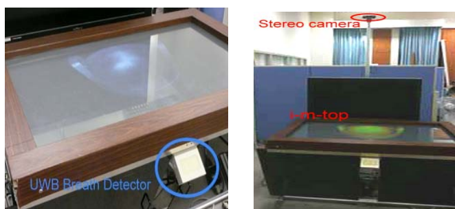
Fig. 1. (a) The architecture has the UWB Breath Detector set underneath the Interactive Multi-resolution Tabletop (i-m-Top). (b) The architecture is composed of a stereo camera and an Interactive Multi-resolution Tabletop system.
