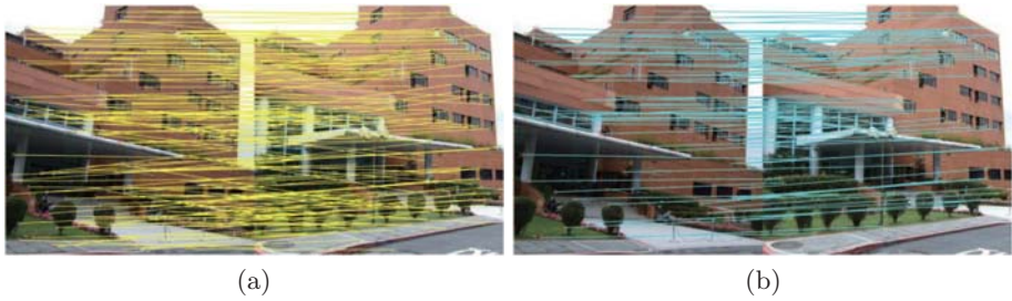
Fig. 1. (a) Two frames showing the same building from different camera view points, with feature points extracted by Harris corner detection, and their correspondences, and (b) final geometrically consistent points as evaluated by the RANSAC algorithm
