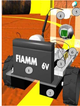
Fig. 4. The prototype of SNFRbot: 1) 6V battery, 2) motor driver, 3) microcontroller, 4) video cam, 5) heat sensor, and 6) gas sensor
