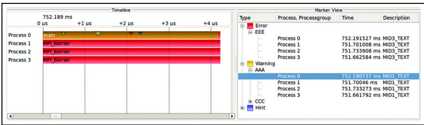
Fig. 2.5: Performance markers highlight hot spots during the execution of a program. Individual markers can be selected in a hierarchical list (right). Their occurrence in time is depicted as colored triangles in the respective timeline views (left).
