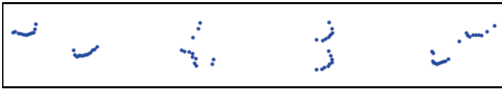
Fig. 8.1 Typical range readings from legs of people. As can be seen, the appearance can change drastically, also because the legs cannot always be separated.
