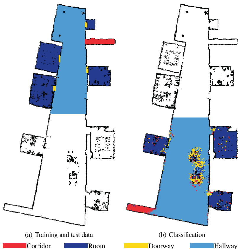
Fig. 3.11 (a) Training data ( colored ) and test data ( white ) from the environment with four classes. (b) Classification results after applying the decision list corridor-hallway-doorway to the test set.
