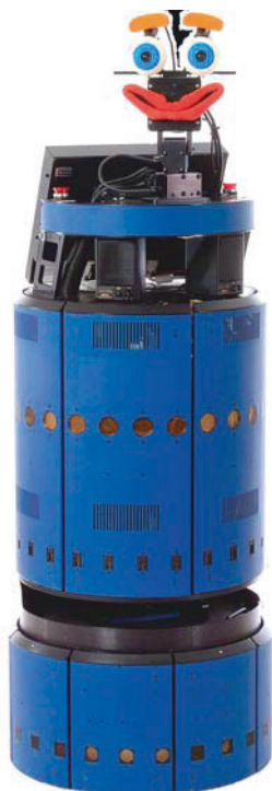
Fig. 5.4 The image shows the robot Albert which was used for the experiments. Albert is a B21r robot equipped with a SICK laser range finder and a camera system mounted on a pan/tilt unit.
