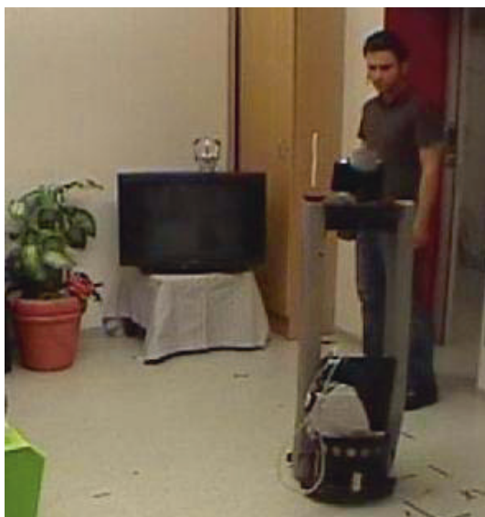
Fig. 7.9 Following the order “go to the television”, the robot approaches the navigation node from where it saw the television set the last time.
