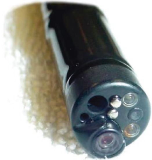
Fig. 112.16 Tip of confocal endomicroscope revealing laser imaging portal
