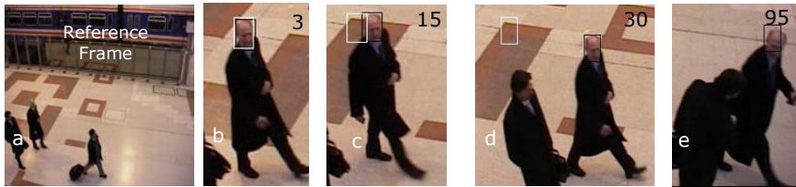
Fig. 3. A comparison of the proposed CWT tracker (indicated with black box) with MS tracker (represented by white box) on PETS 2006 video dataset S1 (camera 3)
