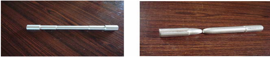
Fig. 3. Tensile specimens (Before & after test)
