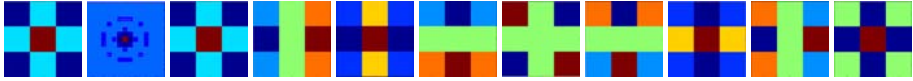
Fig. 2. The set of new filter used for the current experiment. Filter 2 is the new omni-directional high pass filter changed. (The first low pass filter is used twice on two different color channels which gives a total of 12 features.)
