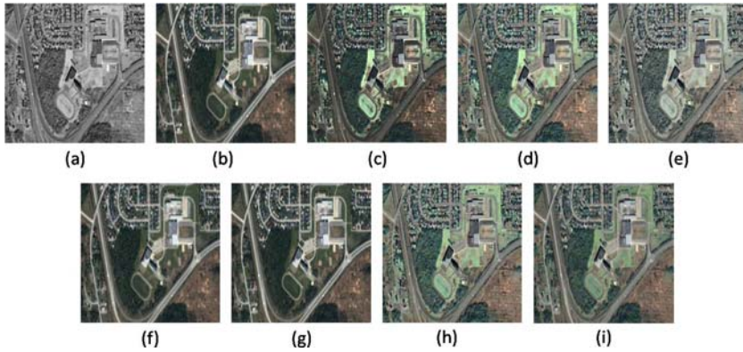
Fig. 3. Fusion Results of IKONOS2 image (a) 1m Panchromatic image (b) 4m Multispectral image (c) IHS Method (d) Modified IHS Method (e) PCA method (f) WT method (g) CT Method (h) Brovey Transform Method (i) Proposed Method
