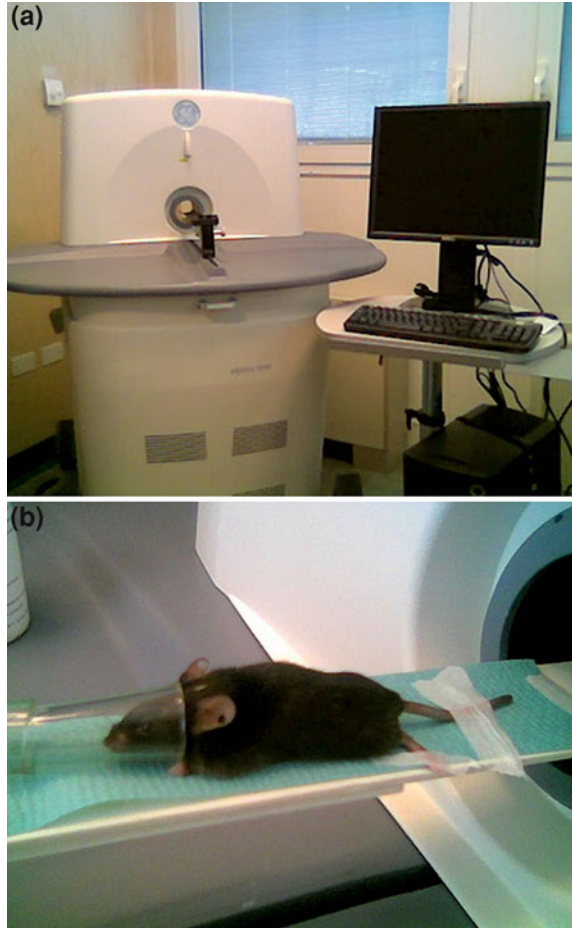
Fig. 1 a Small animal PET tomograph. b An animal model of cancer during gas anaesthesia on the scanner bed
