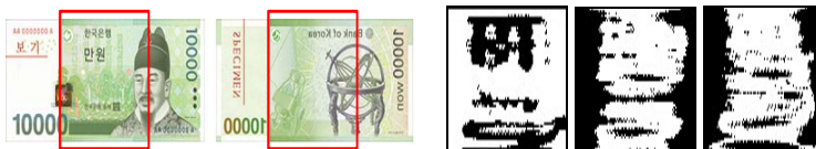
(a) Area of banknotes used for experiment (b) Images obtained by UV sensor
