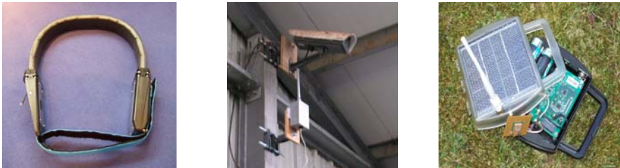
Fig. 3. (a) A collar with antenna diversity; (b) An installed base station at the farm; (c) Solar powered router with antenna diversity.
