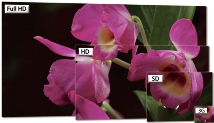
Fig. 2. Typical resolutions for standard video formats
