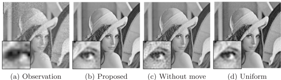
Fig. 3. Comparison of estimation results when the series of observed images suffer from the occlusions shown in Fig. 1. (a) One of the fifteen LR images. (b) Proposed (30.69 dB). (c) Without movement (29.13 dB). (d) Assumed uniform noise (28.66 dB).
