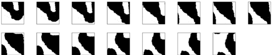
Fig. 1. The binary occlusion patterns (black: large noise of 10 dB, white: small noise of 40 dB). The occlusion patterns were shifted according to \boldsymbol{\theta} .
