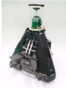
Fig. 1. “Musashi” robot includes an omni-directional platform, an omni-vision, and strong novel ball-kicking device, laptop PC and 90 [W] motor, omni-directional wheels and batteries
