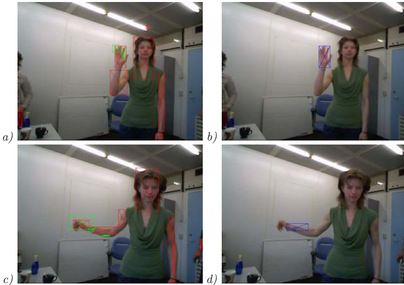
Fig. 2. Marked regions of interest. Red and green areas denote skin and motion area, respectively. A blue area is the combined moving skin area that has been averaged over all skin areas that are moving.
