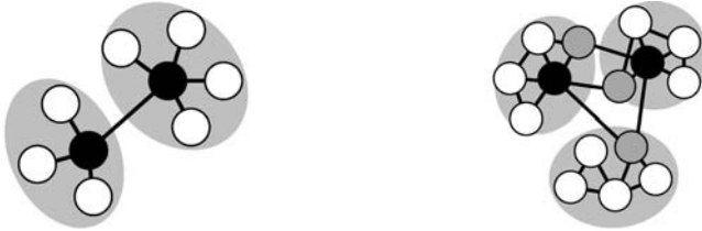
(a) Two nodes from different communities connected by an edge (b) Two nodes from different communities share many common neighbors
