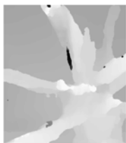
Fig. 4. Example 1 disparity map without the interpolation with stereo parameters 15px for window and 50px for search
