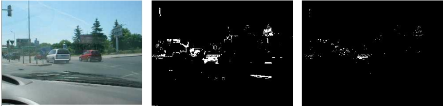
Fig. 5. Car tracking example in a traffic sequence (left). A confidence map with the RGB color components (middle). A confidence map with the IJK and ST components.
