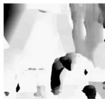
Fig. 5. Example 2 disparity map without the interpolation with stereo parameters 18px for window and 30px for search
