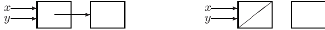
Fig. 4. Snapshots of the heap during the execution of the program in Remark 2. The lefthand side and the righthand side show the states before and after executing *y \leftarrow \mathbf{null} respectively. The rightmost cell will be leaked.
