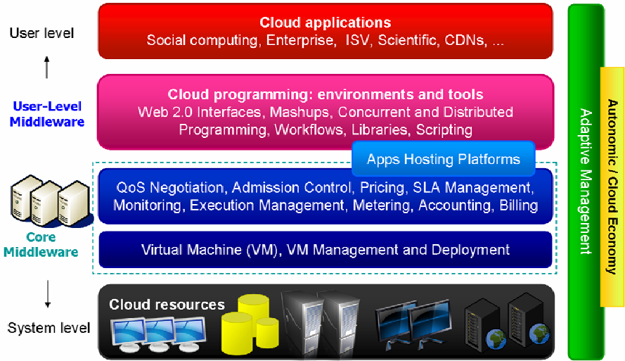
Fig. 4. Cloud computing reference model
