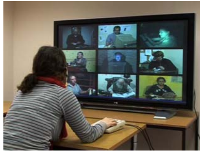
Fig. 1. A user interacts with the Crossed Lines interactive film installation. When a key is pressed on the telephone keypad, an action is triggered on the corresponding screen, and the user listens to the audio through the telephone hand-set.
