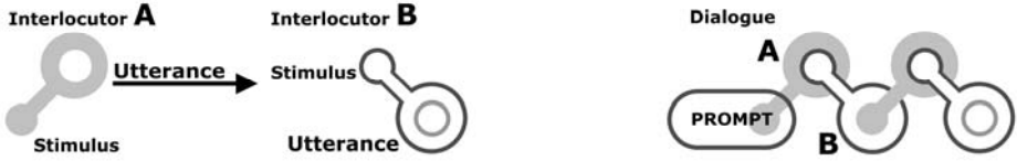
Fig. 2. Interlinking dialogue acts of two interlocutors by connecting a concrete utterance of one bot with a stimulus for an utterance of another one
