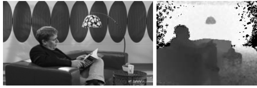
Fig. 1. High resolution color image and corresponding low resolution ToF depth map. Due to the low resolution of the ToF camera the lamp arm is not observed in the depth map although visible in the color image.
