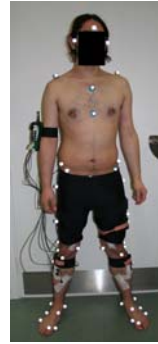
Fig. 3. Motion capture marker setup defined in this study
