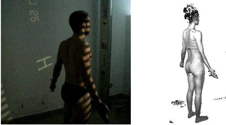
Fig. 1. Left: Breuckmann bodySCAN in action. Right: example of mesh with associated texture. It is possible to notice holes in shadowed and reflective regions.
