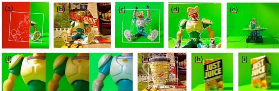
Fig. 7. (a) recognition of significantly occluded objects, (b) object with background clutter, (c) recognition of deformable object, (d-e) examples of scale change, (f) lighting variations, (g) misaligned bounding box with scarcity of cup-handle features, (h-i) blur
