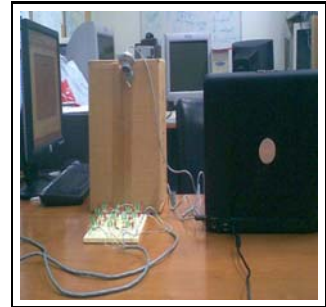
Fig. 4. Experimental setup: Receiver is Web camera, Transmitters are LEDs on Breadboard
