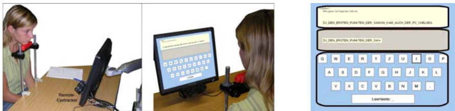
Fig. 1 Left: Experimental setting during the gaze-typing task. A participant is seated in front of the screen that displays the gaze-typing interface. Two miniature cameras of the LC Technologies eye tracker are mounted below the screen and monitor the user's eye movements. Right: Stimulus display screen during a trial. The top frame marks the task area, the middle frame the input control area and the bottom frame the interaction area. Frames are inserted for illustration purposes only and were not visible during the experiment. Some text has already been typed and appears in the input control area. The currently selected character 'I' is marked by a green surround (dotted here for illustration) to provide feedback to the user about the successful selection.
