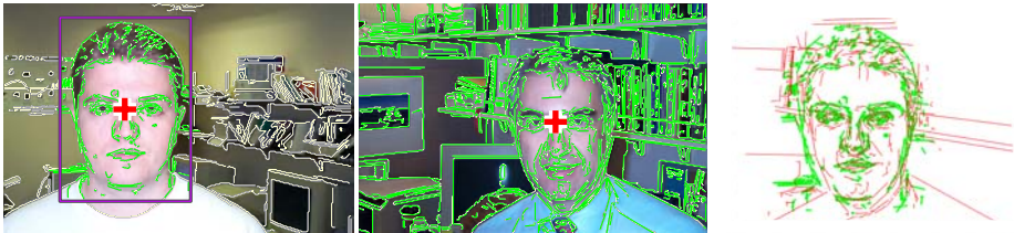
Fig. 3. Example of the object localisation by matching and fitting a noisy model (contents of the bounding box in the left image). The second image shows the features extracted from the target image and the estimated location of the object centroid (strongest voting maximum). The right figure shows the alignment of the model (green, thick lines) with the uniquely corresponding features in the target image (red, thin lines). Note the amount of clutter in the target image.
