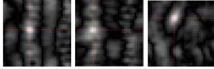
Fig. 2. Ortho-view of a resulting 3D correlation grid in the (\xi, \eta, \omega) -space with a maximum spherical harmonic expansion to the 16th band, \phi = \pi/4, \theta = \pi/8, \psi = \pi/2 . From left to right: xy-plane, zy-plane, xz-plane. Clearly, our fast correlation function obtains an isolated and stable maximum in a single point on the grid.
