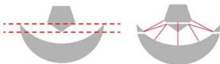
Fig. 2. Step three of the algorithm is invoked, if the convex hulls of the two shapes overlap. Left: The objects are recursively divided into sub-meshes according to support planes (dashed red lines). Right: The minimum of the set of separation distances (red lines) of the sub-mesh pairs gives the separation distance.
