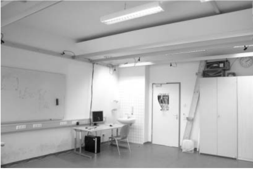
Fig. 2. Lab setup for our real-time 3D reconstruction system. The cameras are mounted on movable profiles to allow an easy reconfiguration of the camera setup.
