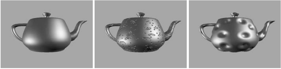
Fig. 1. A teapot with different combinations of materials. From left to right: a simple plastic material, a bump-mapped plastic, and a geometry shader that tessellates and displaces the teapot.
