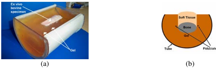
Fig. 10. Quantitative validation experiment. (a) Picture of the constructed phantom, (b) Axial view schematic sketch of the phantom.
