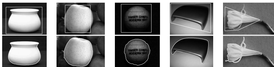
Fig. 4. Segmentation results of the CCLBF model on five real images. Row 1: Original images with initializations of contour. Row 2: Segmentation results of the CCLBF model.
