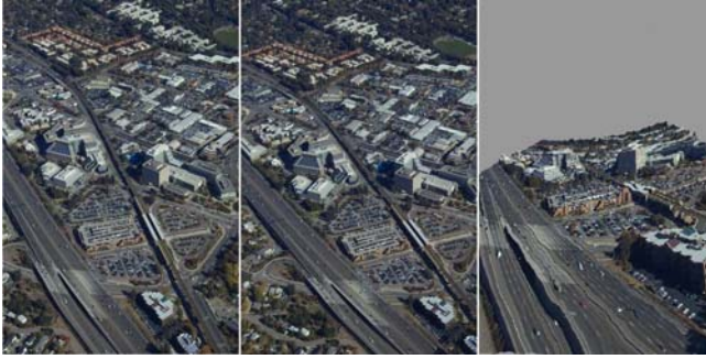
Fig. 2. Aerial source images (left, middle) and the resulting triangulation from a different view point(right)
