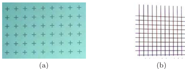
Fig. 3. (a) Camera Image of calibration pattern with plus marks (b) Camera Image of the grid pattern projected onto reference plane to compute homographies (with colours inverted)
