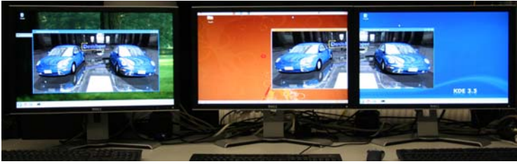
Fig. 5. Real-time ray tracing simultaneously displayed on three presentation hosts, all of which are fully interactive and synchronized. The rendered images are displayed in a single window on one computer (left) and a display-wall via two split video streams on two additional machines (right).
