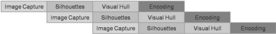
Fig. 3. Reconstruction pipeline on the slave PCs. Each row represents the processing steps taken for each group of simultaneously acquired input images. The processing times are 8 ms, 15 ms, 15 ms and 10 ms respectively. This leads to a very low latency on the slave PCs, which is pushed to about 100 ms when considering image exposure time and computations on the master PC. Due to the pipelining the whole system can run at a frame rate of 30 Hz or higher.
