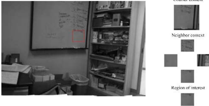
Fig. 1. A sample of the sources of the contextual information in our proposal, i.e. the patches surrounding the ROI at the same scale and the patch at a coarser scale level with respect to the ROI
