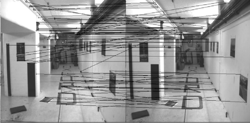
Fig. 2. The first two images of the test sequence Corridor , superimposed with black lines indicating 89 correspondences that were detected by SUSAN [7] feature detectors
