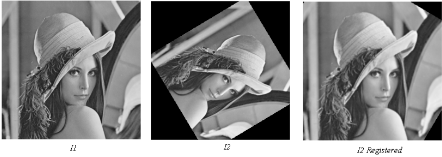
Fig. 1. Image registration. Left: reference image; middle: image to register; right: registered image I_2 .
