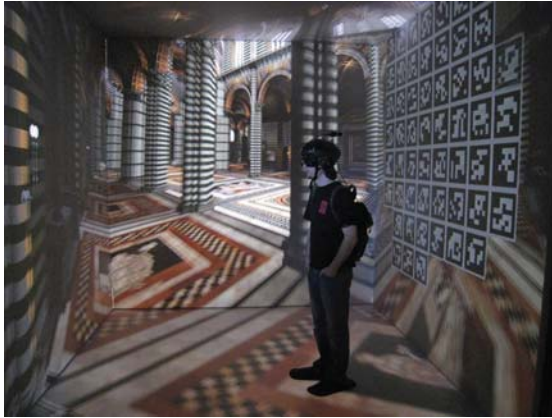
Fig. 1. Example of how fiducials are displayed in the VR space by the original JanusVF. Worn on the user's head, the camera faces exactly opposite the the user's point of view to track fiducials that are displayed on the wall behind the user.
