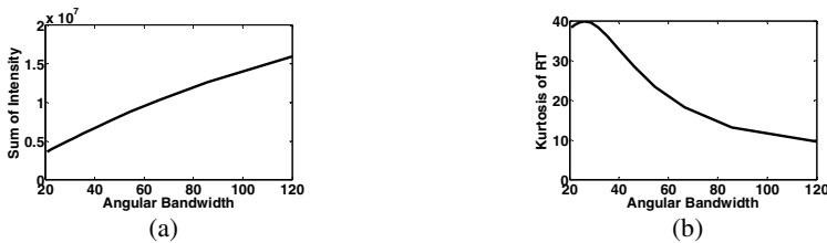
Fig. 9. Angular bandwidth selection. (a) Filter angular bandwidth versus sum of intensity values of A_\gamma . (b) filter angular bandwidth versus kurtosis of RT obtained from calculating the RT of A_\gamma .
