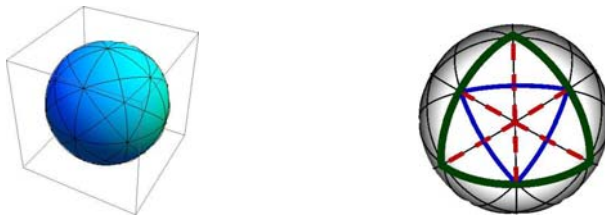
Fig. 5. Partition of the view vectors for a 3D cube. The highlighted portion of the right figure represents a octant.
