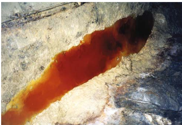
Fig. 8.2 Acid rock drainage solution in the “Himmelfahrt Fundgrube” mine at Freiberg, Germany (length of the puddle: ca. 1 m)
