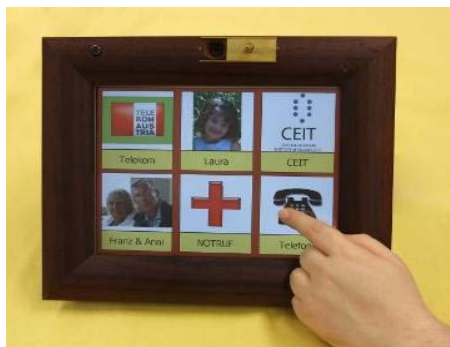
Fig. 1. The final videophone-prototype as it was developed iteratively in the Living Lab. This version was duplicated for use in the field evaluation.
