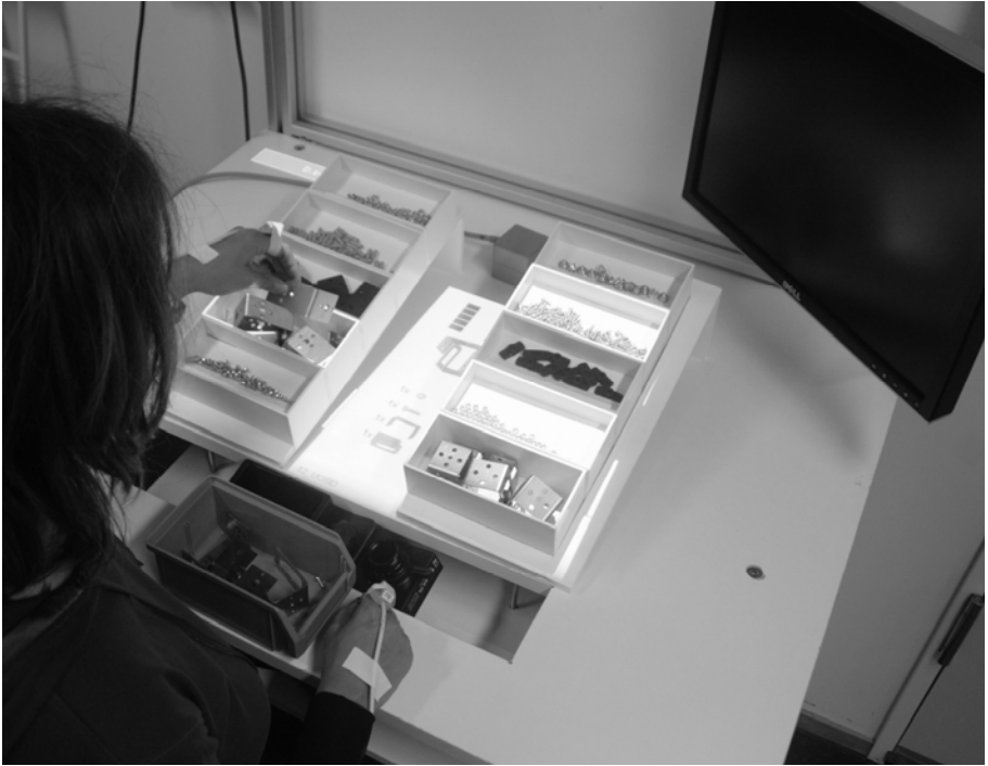
Fig. 2. Experimental setup with the working area, beamer projection, monitor, source of the motion tracker as well as the remote eye tracker. One exemplary participant is selecting and grasping one item with the left hand in order to place it inside the box in front.
