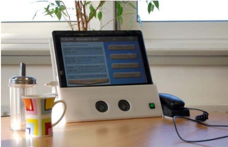
Fig. 1. The Building Bridges device showing the Main Menu Screen: On the Main Menu Screen the user can view the time, day and topic of upcoming broadcasts
