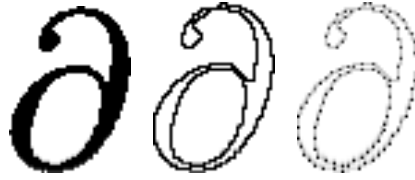
Fig. 2. Process to identify the set P of points in the symbol shape (on the rightmost image)
