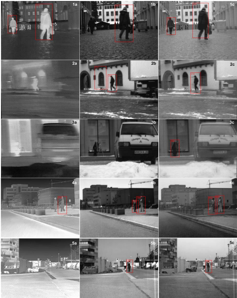
Fig. 4. Examples of the Evaluation Scenes: 1–3: winter scenario, 4–5: summer scenario; a) FIR image b) NIR image c) Fused image
