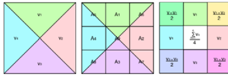
Fig. 4. Correlation between the upper layer cell subparts and the actuators layer cells
