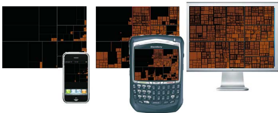
Fig. 1. Example and application of a progressive treemap providing a tour-through-the-data and uncomplex adaptation to a variety of viewing devices
