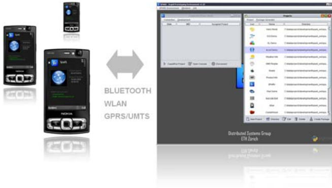
Fig. 1. Multiple mobile phones with the SPARK client software can be connected to a SPARK environment instance running on a PC
