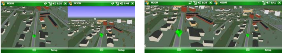
Fig. 3. Left: Speed-dependent camera control based on height angle. (Left: 0-10 km/h; right: 40 km/h or more.) Right: Speed-dependent camera control based on distance (Left: 0-10 km/h, right: 40 km/h or more).
