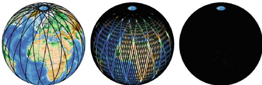
Fig. 3 GOCE orbit on the earth surface after 1 day, 1 week and 1 month mission duration
