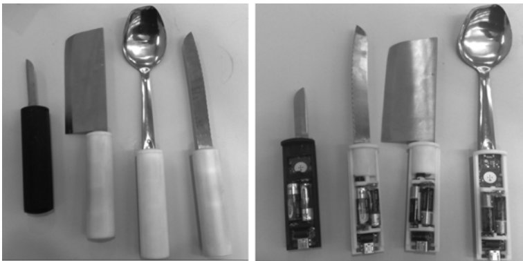
Fig. 1. Modified Wii Remotes embedded in specially designed handles
