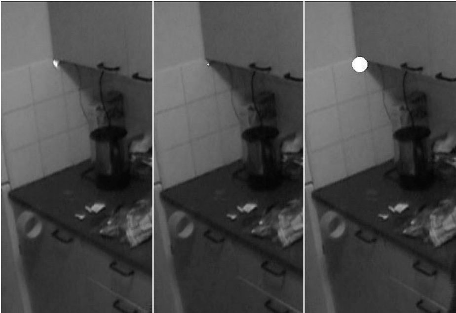
Fig. 2. Video observation of the kitchen, left: an active marker signal as captured by the video camera, middle: selecting the active marker with a dot, right: a reaction on the activated marker
