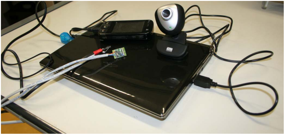
Fig. 5. The prototype of EMon with its components connected: a netbook, a PDA, a webcam and two sensors
