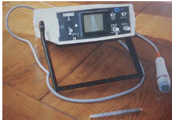
Fig. 28.1 The antique Dymax TM-18. This is the ultrasound unit that we took in 1995 for the Paris-Dakar rally. This machine, with five buttons, no space for storing images, only one probe and a battery, i.e., full autonomy, prefiguring the modern “stethoscope.” The pen in the foreground indicates the size of the machine
