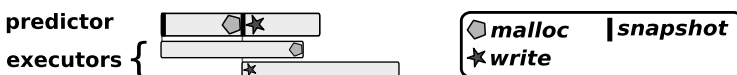
Fig. 2. The temporal order of malloc and the write access are different between predictor and executors. Checks use speculative variables to defer the check of the write .
