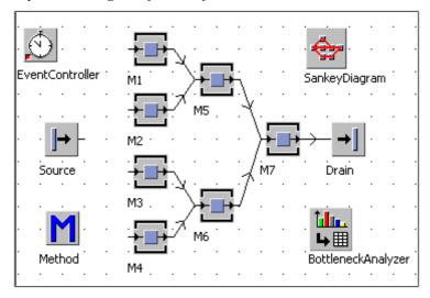
Program the method and assign it as the exit control (front) to the source. The source is to transfer the parts to the first available and operational machine.
