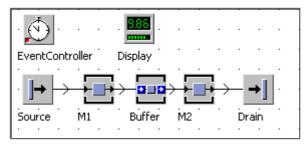
Settings: Source interval: 2:10, M1 processing time: 2:00 availability: 90% 1 hour MTTR, M2 1 minute processing time 50% availability, 2 hours MTTR, Buffer capacity 1,000 no processing time. The display should show the stock of the buffer.
