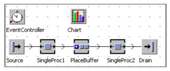
Settings: SingleProc1, SingleProc2 processing time 1 minute each, availability SingleProc1 and SingleProc2 95% MTTR 3 hours, use different random streams, PlaceBuffer capacity 100, accumulating, 30 seconds processing time.
