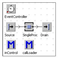
Settings: Source interval 2 minutes, SingleProc 2 minutes processing time, inControl as entrance control SingleProc. The method callLoader writes a short message into the console. Method callLoader:
