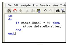
Confirm your changes with  $\checkmark$ . You now have to assign the method to an object. For this purpose, each object has one or more sensors. When an MU pass through a sensor, the relevant method is triggered. Double-click on **STORE – CONTROLS – ENTRANCE**; select the correct method, ready we are!
