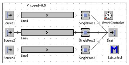
Settings: Source1 to Source3: interval 1 second, not blocking, Conveyors: 12 m, 0.5 m/s, SingleProc: each 1 second processing time, Failures: 90% availability, 10 minutes MTTR, Drain: 0 seconds processing time.
