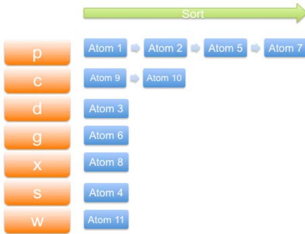
Fig. 1. Example tree data structure that uses a set of priority heuristics to reorder atoms for the sample rule from the California Driver Handbook. The left-hand column (orange boxes) contains variables used in the first position of a SWRL predicate. The atom number (blue boxes) represents the original ordering provided in the SWRL rule.
