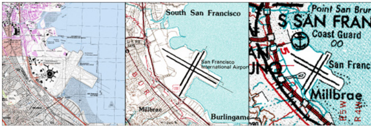
Fig. 3. San Francisco International Airport in USGS Topographic multi-scale map series. Left to right 1:24,000 7.5" Quadrangle, 1:100,000 30' x 60' Quadrangle, and 1:250,000 1 degree by 2 degree Quadrangle, presented as uniform-scale graphics.
