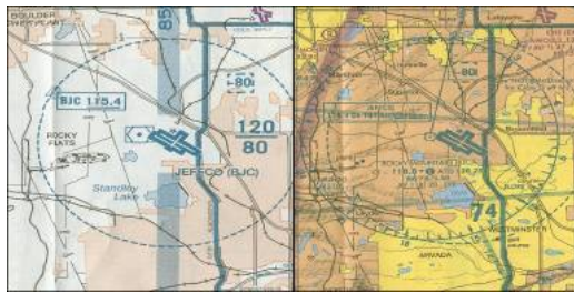
Fig. 2. Section of IFR and VFR Charts over Jefferson County Airport. Two cartographic ontologies based on one spatial database model.
