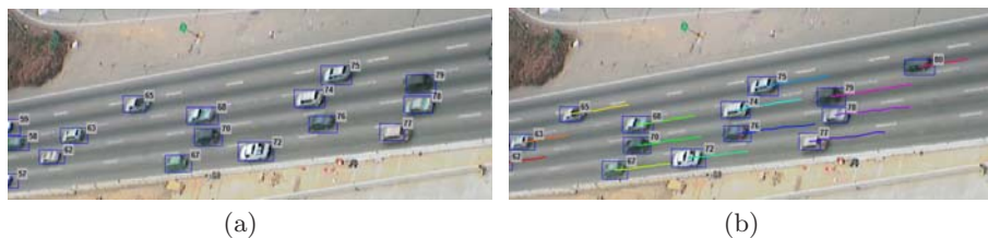
Fig. 1. Two frames (209, 218) of a traffic sequence are viewed in which the objects are identified and tracked
