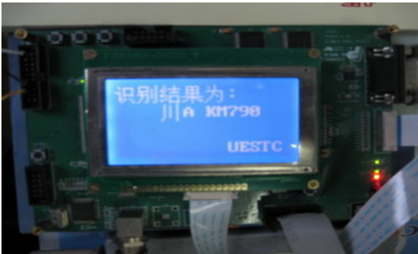
Fig. 8. Recognition result of a license plate
