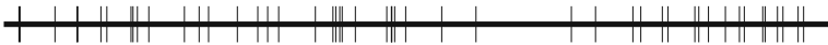
Fig. 4.3 Example of a Poisson process error pattern with constant error rate. Vertical lines mark errors observed over the horizontal time axis
