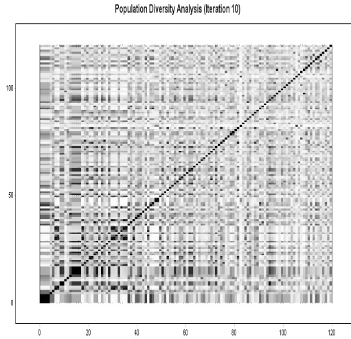
Fig. 2. Degree of similarity/distance for all pairs of solutions in a SGA's population of 120 solution candidates after 10 generations
