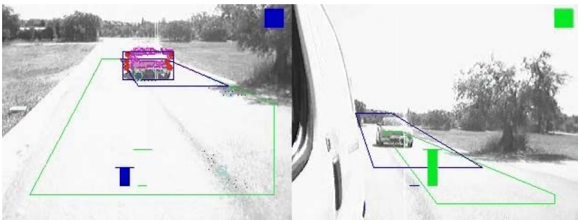
Fig. 8. Panoramic Blind Spot Detection system (Panoramic BSD)
