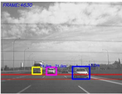
Fig. 7. Left: detected vehicles on a test sequence. Right: filtered y-position of the car located in the middle lane.
