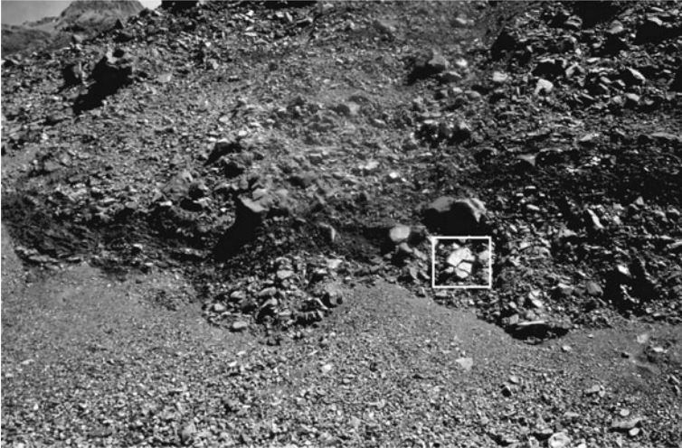
Fig. 19.1 Preserved banding sub-facies at the Falling Mountain rock-avalanche deposit consisting of highly fragmented, angular, fine, bands of dark argillite and highly fragmented, angular, coarse, light coloured greywacke. Highly fractured but relatively undisaggregated clasts are common; a large greywacke example is highlighted. The boundaries between bands are sharp with no evidence of mixing. Height of river-cut exposure is approximately 4 m
