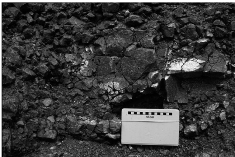
Fig. 19.2 Close up view of a highly fractured but undisaggregated greywacke clast at the Falling Mountain rock-avalanche deposit. Distinct “impact” marks are preserved with fractures radiating away from them. These features must have either been transported without the fractures opening and allowing matrix infill and further fracture as observed in Fig. 19.1; or, this represents a fracture event immediately before the cessation of motion of the rock avalanche
