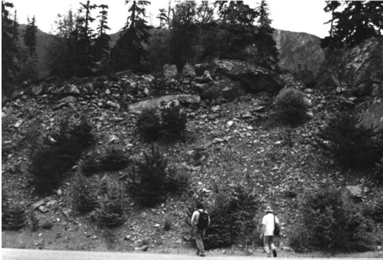
Fig. 17.15 Section through Mystery Creek (Green River) rock-avalanche deposit, showing the finely crushed interior. Dynamic grain fragmentation in the failure of grain bridges is the cause of the comminution. Grain fragmentation imparts a dispersive stress of the magnitude of the Hugoniot elastic limit of the rock material appropriate for the local strain rate and confining stress
